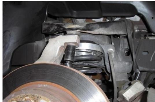
Tighten upper ball joint nut to OEM specifications.
