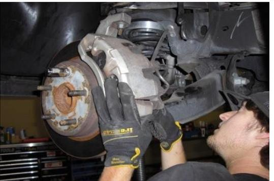
Re-install the brake caliper using the factory hardware. Tighten to factory specifications. Use a thread locker if needed.
