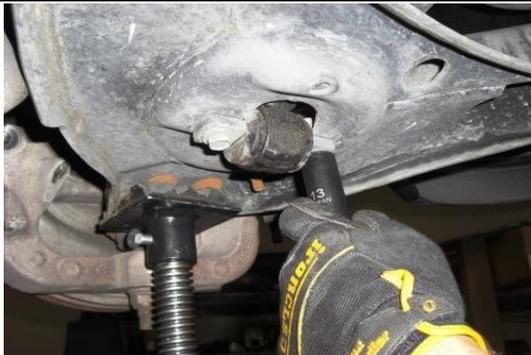
Remove the two lower shock mounting bolts with a 13mm socket. Set aside for later use.
