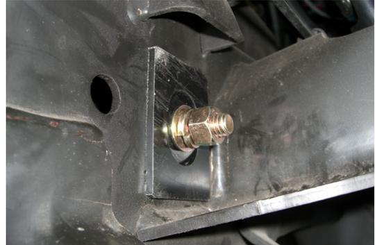
On the backside of the frame rail, install backing plate, flat washer and nyloc nut. Tighten to 85lb-ft.
