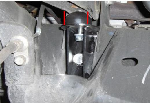
Center bump stop under the recess of the upper control arm. Tighten down the bump stop nut with a 13mm socket
