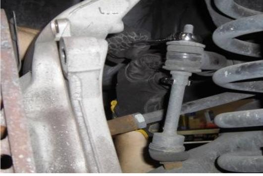
Using a 16mm wrench, remove the upper sway bar nut.
