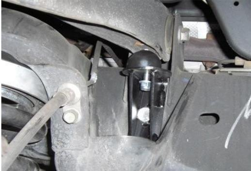
Install bump stop onto driver side bracket but do not fully tighten. Install driver side bracket onto driver side of truck using the M12-1.75x100mm bolt provided.
