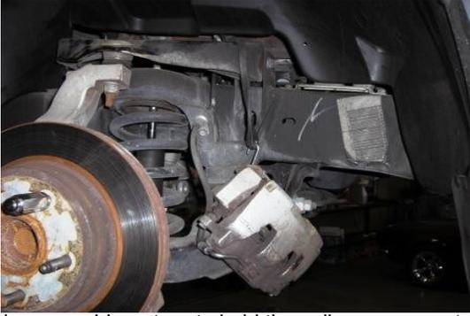
Use wire or a rubber strap to hold the caliper up so as to not stretch or tear the brake line.
