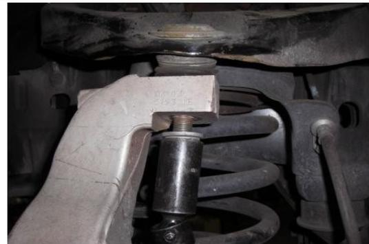
Loosen but do not remove the upper ball joint nut with a 21mm.
