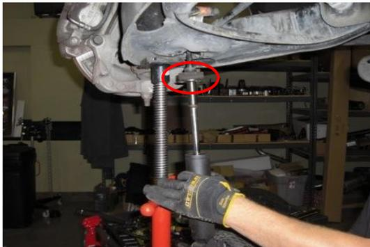
Install the shock stem lower plate and bushing onto extension. Install shock into factory location.
