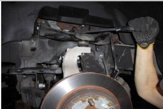
Once suspension is compressed enough use a jack to support it and compress it a little more. Use a pry bar to align the ball joint into the knuckle. Install OEM nut.
