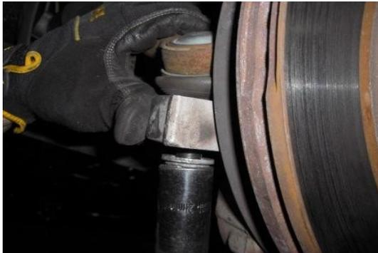
Re-install the tie rod and tighten to OEM specifications.
