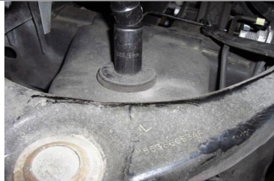
Remove the upper shock mounting nut using an 18mm socket. Set the nut, bushing, and plate aside.
