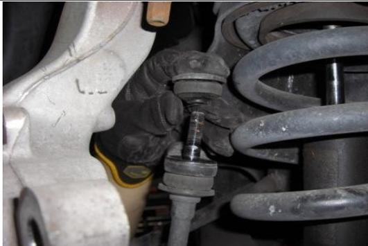
Remove the bushing and bushing plate. Set it aside with the nut.
