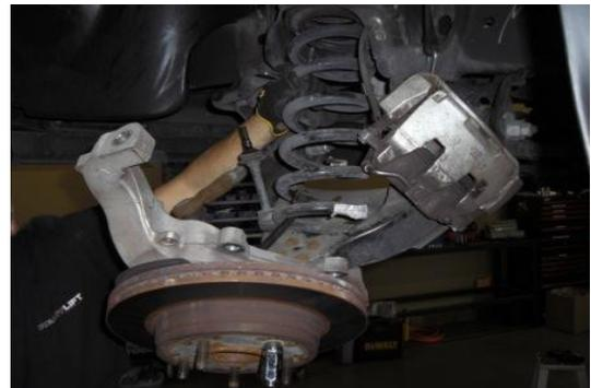
Slowly lower the jack until you can remove the coil spring safely.
