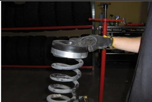
Remove the factory rubber isolator. Place the ReadyLift coil spacer on top.
