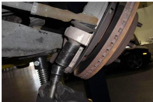
Remove the tie rod nut with a 21mm. Use the proper tool to break the taper.
