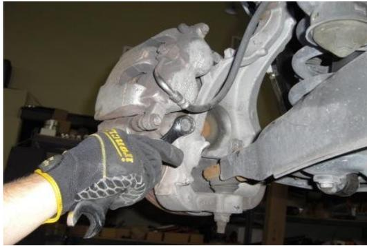
Remove the driver side brake caliper using a 19mm wrench.
