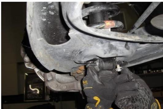
Install the two lower shock mount bolts and tighten to factory specifications.
