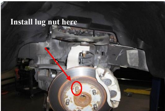
Remove the front wheels. Install one lug nut on each side to prevent the brake rotor from falling off during installation.
