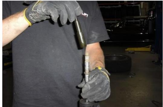
Install the ReadyLift shock stem extension. Be sure to use a light duty thread locker to prevent the extension from unthreading.
