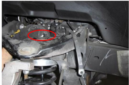
Install the upper bushing, plate, and nut. Tighten to factory specifications.
