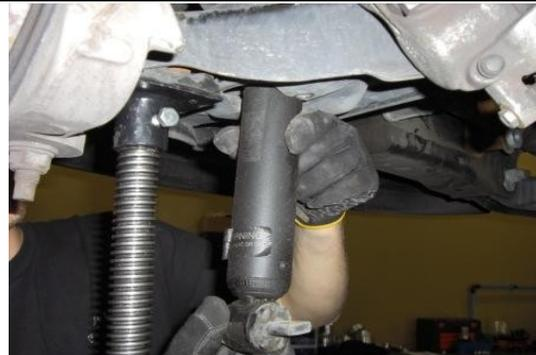
Remove the shock from the vehicle. Remove the upper bushing and plate off the shock stem.
