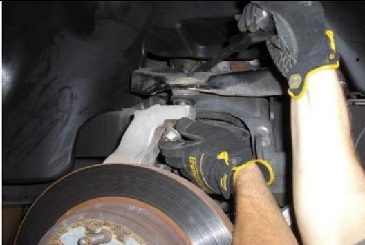
Use the proper tool to break the taper on the upper ball joint. Support the LCA with a jack. Use a pry bar to pull down on the UCA and remove the nut.
