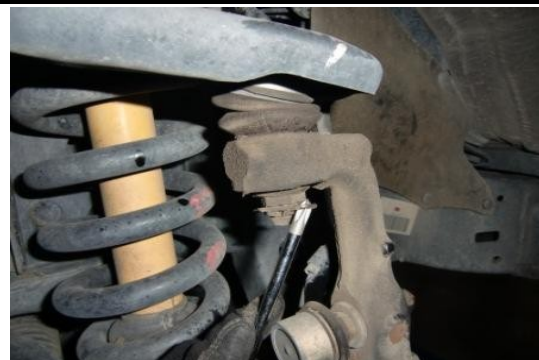
Remove upper ball joint nut retaining clip.
