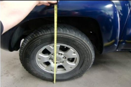
Begin by placing vehicle on level working surface and take an initial measurement.
