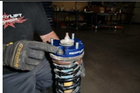
Photo shows factory hardware installed and tightened to factory spec.
