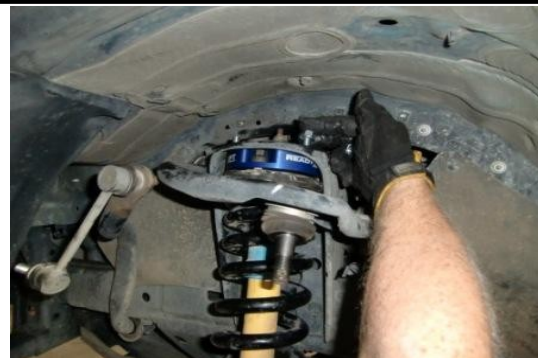
Attach coil-over assembly at the top with provided hardware and torque to factory specs. Reattach all removed hardware in reverse order and secure vehicle on ground.
