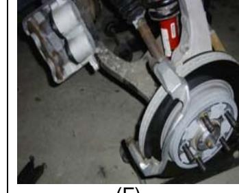
Also remove the brake caliper and secure it as to not overstretch the rubber brake line. (Insert F)
