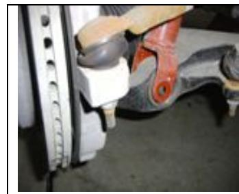
Loosen and remove the upper ball joint nut. Separating the ball joint from the spindle may require the use of a hammer or gear puller if available. Once separated remove the strut from vehicle. (Insert E)
