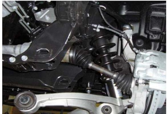
6 ) Reinstall the lower control arm bolts, cams, and nuts, but do not tighten.
