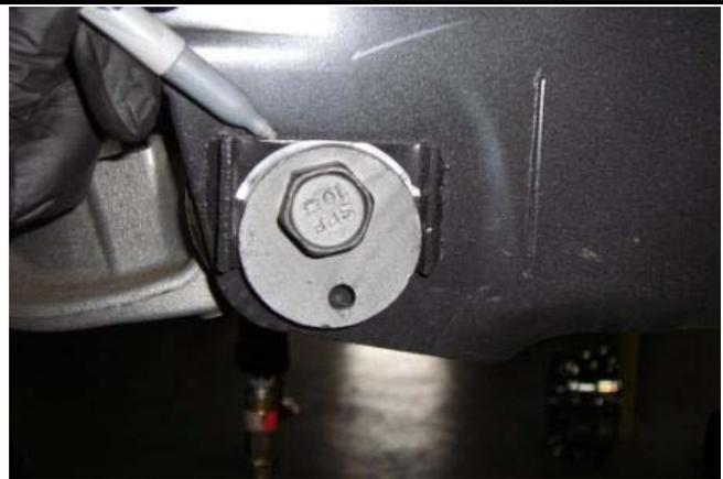
3) Remove the 24mm lower control arm nuts and bolts.
