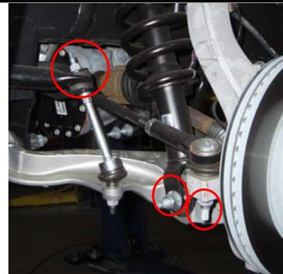
2) Mark the position of the alignment cams on the lower control arm with a marker.
