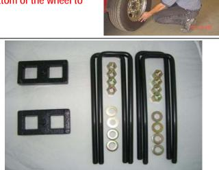
3. Using a jack and a block of wood, carefully raise the truck by the leaf spring until there is enough room for the new block. Install the ReadyLift® 1" rear block.
