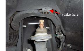
Use a ball joint separator or other appropriate tool to break the ball joint loose from the upper control arm. If tool is unavailable to you, taper can be freed by striking the upper control arm with a hammer. Lower the lack.
