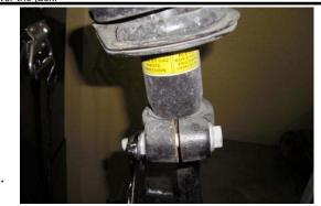
Loosen, but do not remove the strut arm pinch bolt. This allow this strut to rotate around for reinstallation.
