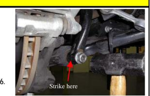
Use a pitman arm puller of similar tool to break the taper. If not available, you can use a hammer to free the taper by striking the lower strut mount while prying on it.
