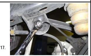
Starting in the driver side, unbolt the upper sway bar end link.
