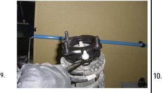
Place the lower strut mount in a vise. Install the ReadyLift strut extension using the factory nuts. Tighten to 42 ft-lbs.
