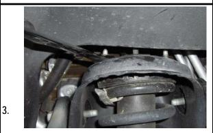
Loosen, but do not remove the two upper strut mounting nuts.
