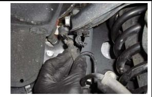
Remove the front wheels. Starting on the driver side, disconnect the ABS line from the support bracket at the knuckle.
