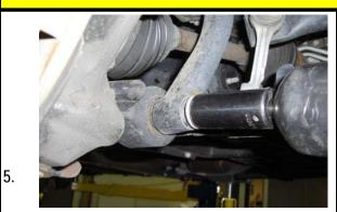
Loosen but do not remove the lower strut mounting nut.
