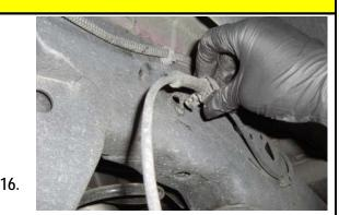
Unclip the ABS Line from the frame rail on both sides. Use a jack to support the rear axle.
