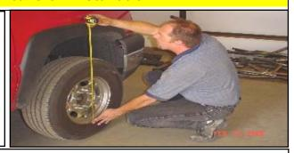
Position truck on a flat surface and lift vehicle by the frame so that the front wheels are off the ground. Use a floor jack and jack stands or a (2) two post lift if available and remove both front wheels.
