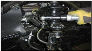
**3**. Remove ABS bracket bolts on the knuckle and upper a-arm.
