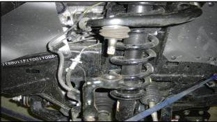
4. Remove the cotter pin and loosen but **Do Not Remove** the upper ball joint nut. Use of a hammer
