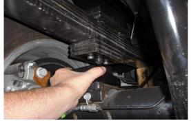
Install the ReadyLift® 1" rear block. Lower the jack and make sure that the leaf spring center pin goes into the hole on top of the block.
