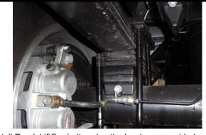
Install ReadyLift® u-bolts using the hardware provided. Torque to 120 ft/lbs. Repeat on opposite side.
