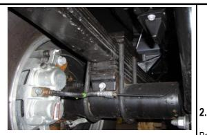
**REAR BLOCK INSTALLATION**Remove the four 24mm nuts.
