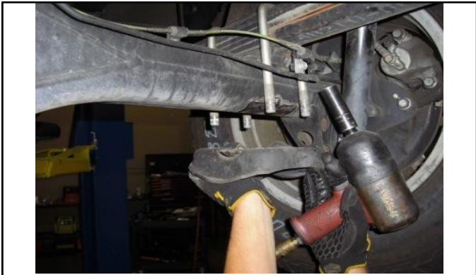
Remove u-bolt nuts and lower plate.
