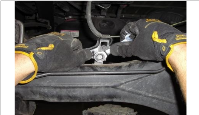
Replace shock on mount and ABS line to axle.
