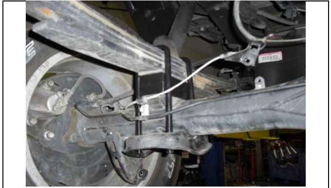
Attach lower mounting plate with provided hardware.
