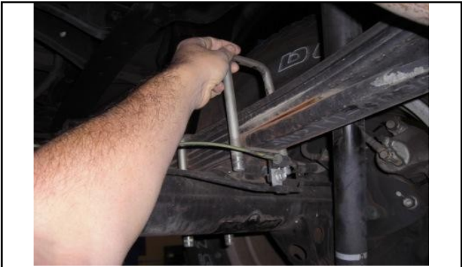
Carefully lower axle and remove u-bolts
