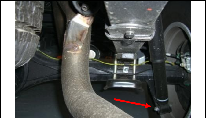
Remove rear lower shock bolt and disconnect shock.
