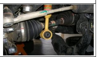
3. Loosen, but do not remove the 19mm lower control arm nut and bolt, Remove the 19mm lower ball joint bolts.
