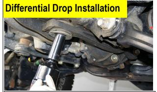
1. Position a floor jack under the front differential. Raise the pad so that it is touching the diff.
