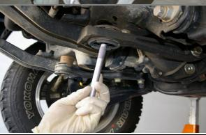
2. Remove the factory 19mm differential mounting nuts and bolts. The OEM washers will be reused.
