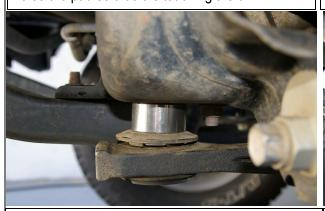
3. Install the 1" spacers between the differential supports and the front cross-member. Install the new bolts with factory washers and the new nuts and washers. Torque to factory specs.
