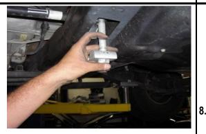
Remove the torsion bar adjusting bolt and nut.
