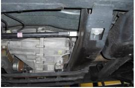
With the vehicle properly secured on a two post lift or Jack and jack stands, locate the torsion bar cross member.
