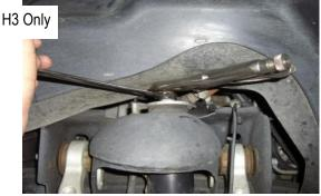
Use a 15mm Wrench and a vise grip to remove the upper sshock mounting nut. Remove the upper bushing and plate.
