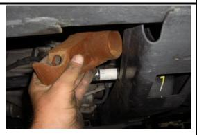
Remove the torsion key.
