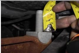
Measure the amount of thread is past the nut on each side. This will be your starting point with the ReadyLift key.
