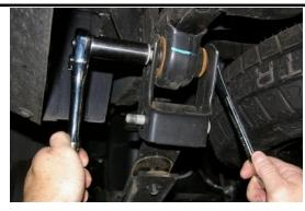
Remove the 21mm upper and lower shackle nut and bolts.
