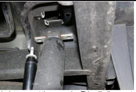
Use a jack to support the rear axle. This will allow you to raise and lower the axle during install. Unbolt the 13mm upper shock mounting bolts.
