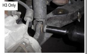
Remove the lower shock mounting nut and bolt. Remove the shock from the vehicle. Remove the lower shock bushing and plate.
