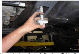
Install the torsion key adjusting bolt and nut. Tighten the bolt so the same amount of threads are protruding past the nut as when you measured.
