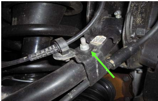
47. Attach the ABS/brake line bracket to the upper control arm.
