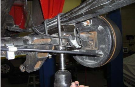
53. While supporting the axle, remove the u-bolts from axle.
