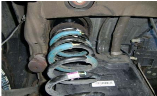
69. Re-install the isolators and coil springs and raise axle.
