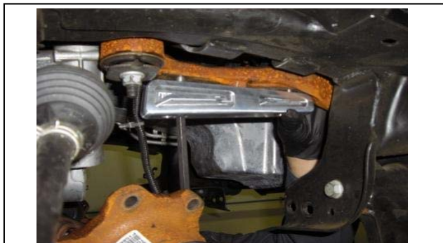
32. Attach both sides with the socket head hardware.
