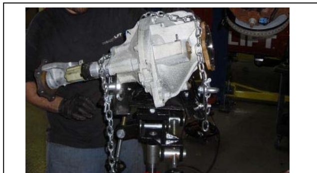
26. Secure the differential to perform the modification.
