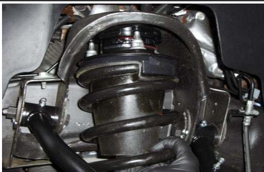
41. Re-install the strut assembly with the new hardware.
