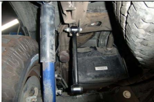
71. Install the new longer sway bar end links and tighten.
