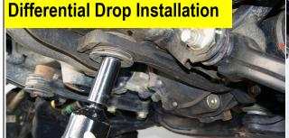
1. Position a floor jack under the front differential. Raise the pad so that it is touching the diff.
