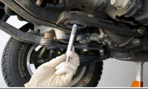
2. Remove the factory 19mm differential mounting nuts and bolts. The OEM washers will be reused.
