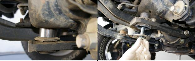
3. Install the 1" spacers between the differential supports and the front cross-member. Install the new bolts with factory washers and the new nuts and washers. Torque to factory specs.
