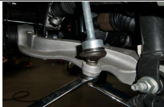
Disconnect sway bar endlinks from below on both dr./pass. side of vehicle as shown.
