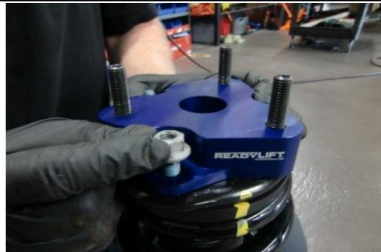
Place spacer on top of OE coil-over assembly and attach with factory hardware.
