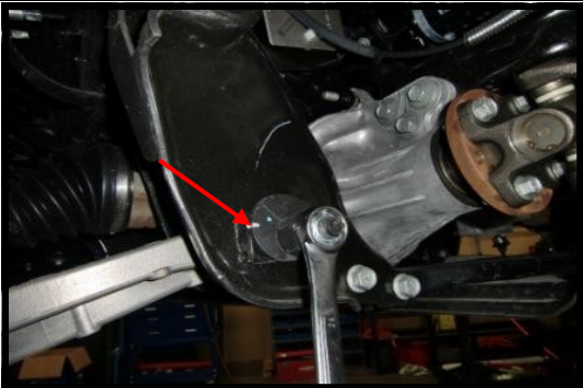
Mark alignment cams on lower control arm bolts before loosening. This will allow additional suspension droop.
