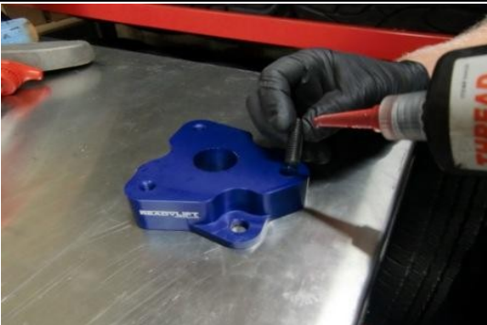
Apply thread locking compound to allen set screws and tighten.
