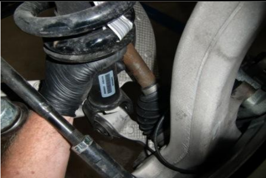
Photo: Lower coil-over mount at lower control arm.
