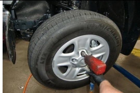
Support vehicle on jack stands and remove front wheels/tires
