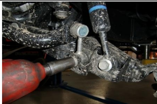
Disconnect sway bar endlinks from below on both dr./pass. side of vehicle as shown, and move bar up
