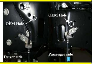
Be sure to double-check that all hardware has been tightened and torqued to factory specs. Remount wheels and tires and torque to factory specs. Re-torque wheels after 25 miles. \*See next page for Tire/wheel fitment specifications.
