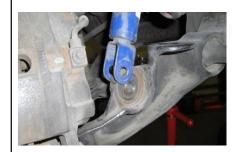
Install the Readylift Shock extension onto the shock using the hardware provided. Tighten to 100 lb-ft.
