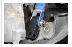
Compress and rotate the shock so the head of the bolt provided is facing towards the frame. Install the shock extension to the lower control arm using the factory hardware. Tighten to 100 lb-ft.
