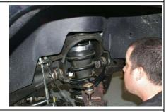
14. Place a jack under the lower control arm and raise it up. Then place the new ReadyLift lower strut mount spacer over the factory control arm holes as shown.
