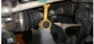
3. Loosen, but do not remove the 19mm lower control arm nut and bolt, Remove the 19mm lower ball joint bolts.
