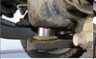
3. Install the 1" spacers between the differential supports and the front cross-member. Install the new bolts with factory washers and the new nuts and washers. Torque to factory specs.
