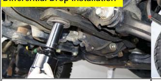
1. Position a floor jack under the front differential. Raise the pad so that it is touching the diff.
