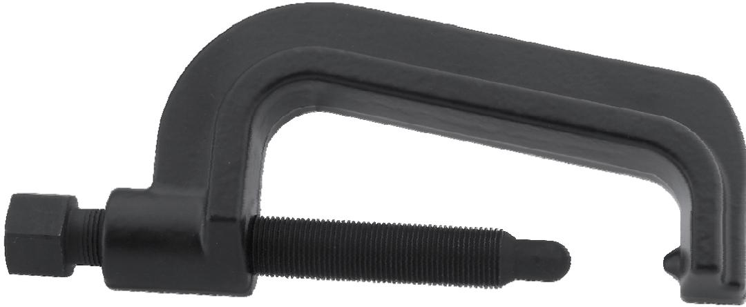
**GREASE BEFORE USE.** Completely remove the threaded bolt and thoroughly grease the inside threads of the tool with high quality Black or Red Molybdenum. Repeat as needed, or after use on four vehicles (eight torsion keys). Remove all metal shavings from the tool threads before re-greasing.
