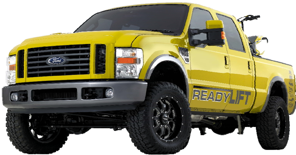
2008 Ford F-250 4WD with RL Part#69-2538 3.5" kit 35x12.5R20 on 20x9 5"BS BMF Wheels Novakane 8
