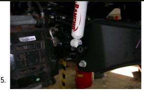
Use a 18mm socket to remove the lower shock mounting bolt on both sides.
