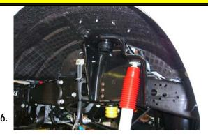
Carefully lower the axle and remove the coil.
