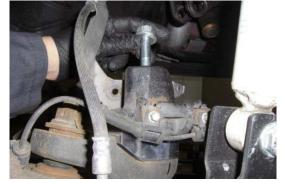
Install the supplied M14 x 70mm bolt and washer through the OEM spring perch and 1" spacer. Tighten to 136lb-ft.
