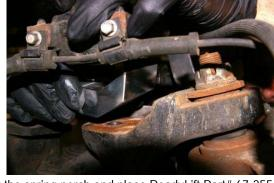
Lift the spring perch and place ReadyLift Part# 67-2551 1" spacer below it.
