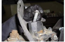
Remove the 18mm spring perch bolt.
