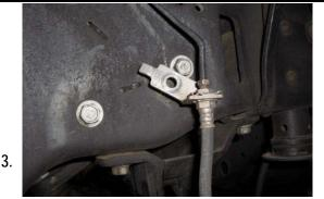
Remove the upper brake line support bracket bolt with a 13mm socket on both sides.
