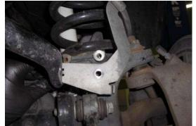
Remove the lower brake line support bracket bolt with a 10mm socket on both sides
