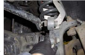
Use a jack to support, raise and lower the front axle. Use a 21mm and 18mm wrench to remove the upper end link bolts.
