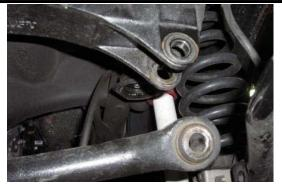
Remove the front wheels. Use a 30mm socket and wrench to remove the upper track bar bolt.
