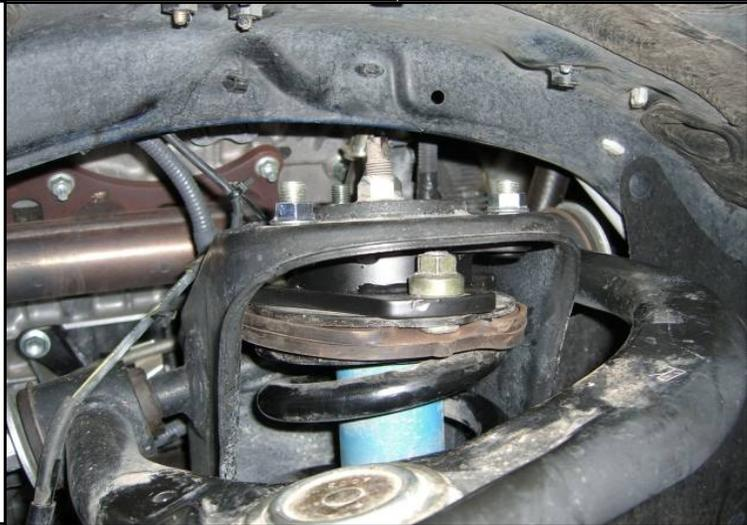
8. Repeat steps 1 through 3 on the Driver's Side of the vehicle. Then re-install the sway bar nuts and bolts on both sides after the upper ball joints have been re-attached. Follow each step closely, making sure to double-check the torque on all fasteners.
