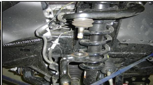
4. Remove the cotter pin and loosen but **Do Not Remove** the upper ball joint nut. Use of a hammer
