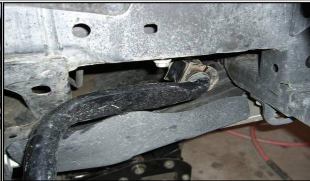
2. Remove bolts holding the front of the sway bar.
