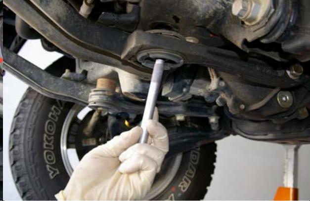
10. Remove the factory 19mm differential mounting nuts and bolts. The OEM washers will be reused.
