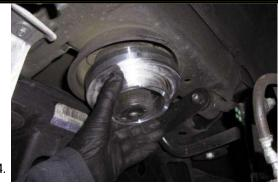
The Readylift rear coil spacer will mount in the factory coil bucket.
