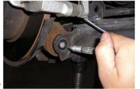
Use a jack to raise the lower control arm, align the mounting holes and install the OEM bolt. Tighten to 117 lb-ft.
