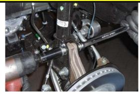
A 24mm wrench and socket will be needed to remove the lower strut mounting bolts.
