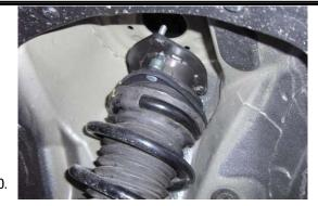
Install strut back into factory location, install nuts supplied with kit but leave loose.
