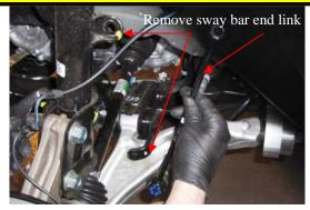
Unbolt and remove the front sway bar end link. You will not reuse this part.
