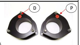
Please note that the ReadyLift strut extensions are driver side and passenger side specific. Arrow points toward front of vehicle
