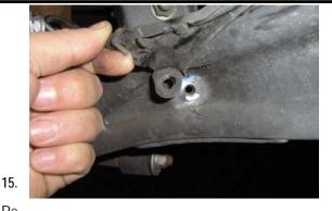
Remove the two 10mm bolts that hold the ABS line support
