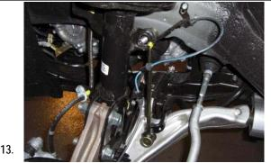
Install the supplied sway bar end link. Tighten to 85 lbft. Reinstall the brake line support bracket and ABS line support bracket using the OEM hardware.
