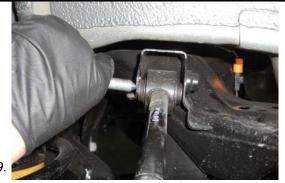
Remove the bolt on the body end of the arm and remove the stock arm. Make sure that both ends of the EZ Arm have equal thread showing on both sides of the turnbuckle.
