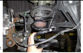
Lower the jack then remove the coil. Be sure to mark where the spring seat is on the lower control arm. You may need to loosen the cam bolt at the frame.
