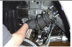
Carefully remove the strut from the vehicle making sure not to drop it on the outer CV boot. Tilting the knuckle towards the rear of the vehicle will make removal easier.
