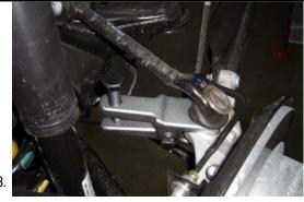
Remove the nut and cotter pin from the outer ball joint end of the upper arm and break the taper using a tie rod end separator.
