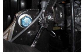
Use a 10mm wrench and remove the ABS line support bracket bolt.
