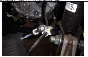
Remove the brake line support bracket using a 12mm wrench.
