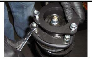
Install the Readylift strut extension using the OEM hardware. Tighten to nuts to 30 lb-ft.
