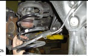
Push down on the lower control arm and install the coil. Make sure that the coil is properly seated in the lower control arm.
