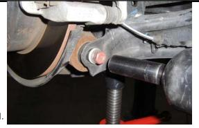
Remove the bolt that connects the lower control arm to the knuckle.
