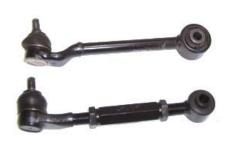
Adjust the EZ Arm to the same length as the stock arm. Install the arm by first installing the bolt at the body, but DO NOT TIGHTEN. Install the ball joint end into the knuckle using the OEM nut and cotter pin.
