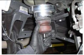
Reinstall the bump stop and bracket with the Readylift coil spacer on top.
