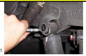
Support the lower control arm with a jack. Remove the rear upper shock mounting bolt.
