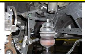
Use a 14mm socket and extension to remove the rear bump stop bracket.
