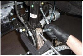
Insert the knuckle into the lower strut mount. A C-Clamp may be needed to align the mounting holes. Insert the OEM hardware and tighten to 200 lb-ft.
