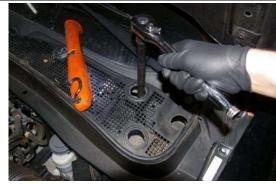
Use a flat screwdriver to remove windshield wiper access panels. Remove the three 14mm upper strut nuts
