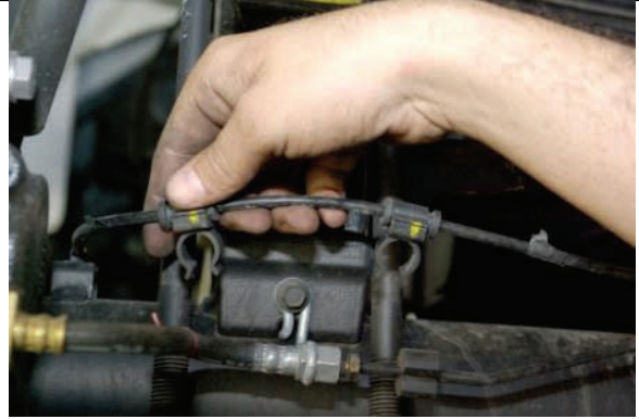
Vehicles with ABS/TC remove clips from U-bolts.
