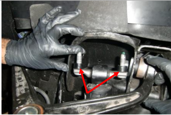
Picture shows spacers being installed onto upper studs.
