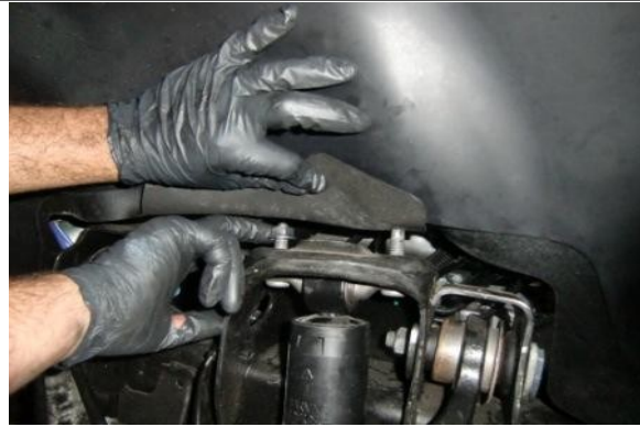
Reposition shock back into frame and tighten to factory spec. using new mounting nuts provided
