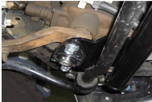
Coat the sector shaft extension with anti-seize. This will allow future removal easier. Install the M12 bolts from the top, then the bearing assembly, washer, and nyloc nut.
