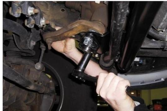
Tighten the assembly hardware so that it is snug. Then tighten the sway bar mounting bolts to 40 lb-ft. Make sure the inner bearing surface can rotate around the sector shaft.
