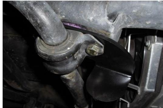
The stabilizing bar will mount against the frame, then the sway bar will swing up and install on top of the stabilizer bar. Use the M10 flange bolts to fasten to frame.
