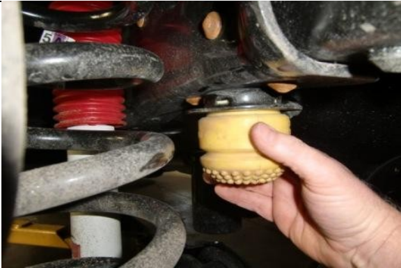
Remove bumpstop and unbolt bracket from frame.
