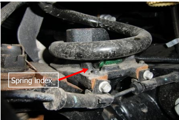
Raise axle and clock coil spring on lower mount as shown .
