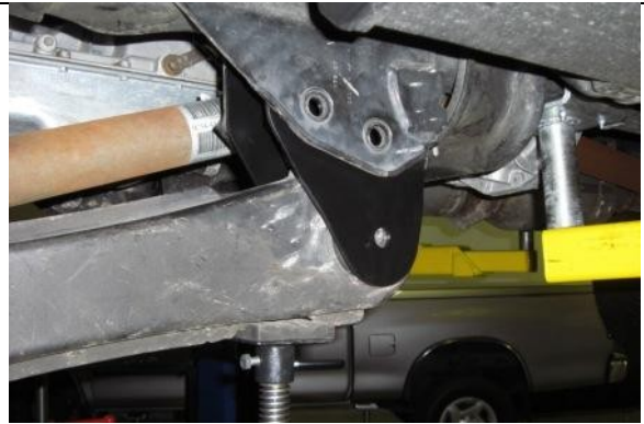
Align bracket with holes in frame and raise arm into bracket.
