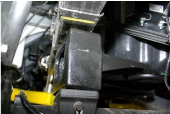
Lower axle enough to install taller block, align and raise axle
