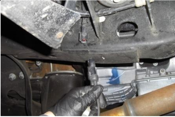
For radius arm bracket option on 3.5 lift kit unplug ABS line.
