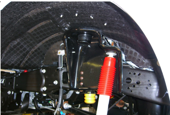
Carefully lower front axle and remove front coil springs.
