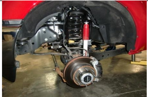
Remove front wheels and tires.
