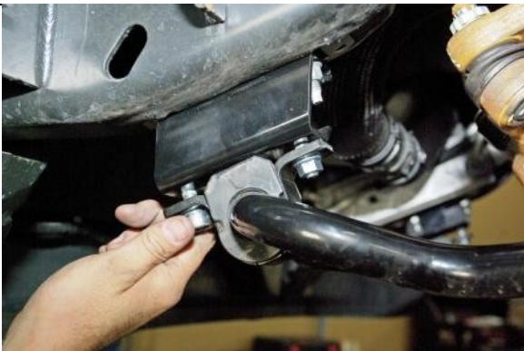
Raise sway bar and attach with new hardware. Leave loose
