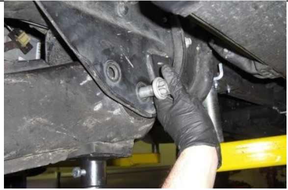
Support radius arm and remove attachment bolts
