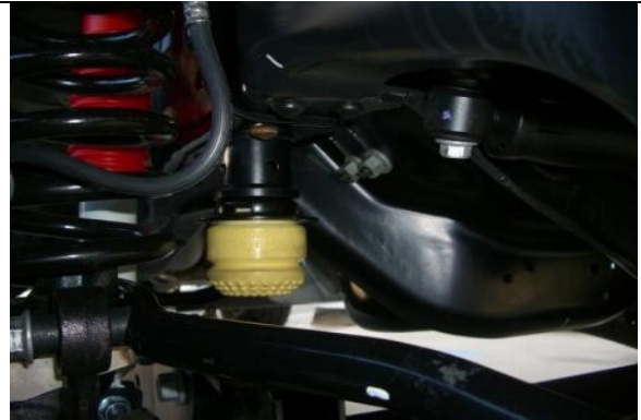
Assemble bumpstop bracket to extension and reinstall.
