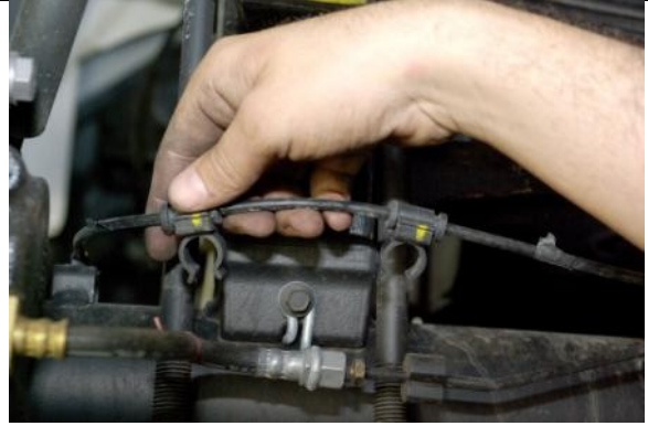
Vehicles with ABS/TC remove clips from U-bolts.
