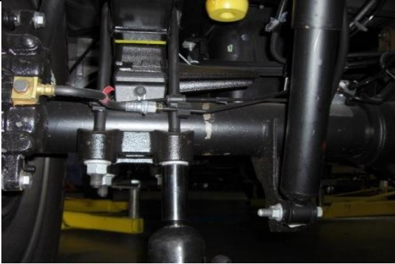
Remove U-bolt nuts and axle mounting plate.
