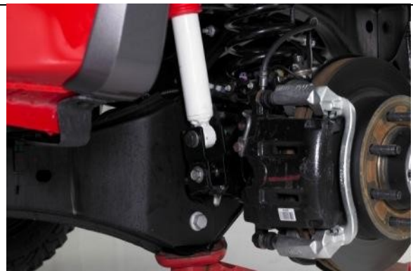
Install and tighten lower shock extension bracket and shock
