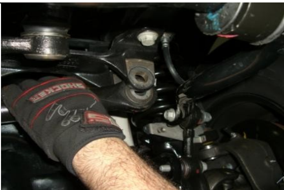
Re-attach trac bar to frame mount and torque to spec.
