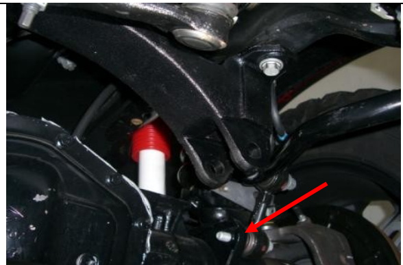
.(05-10) Re-attach and tighten sway bar end links.
