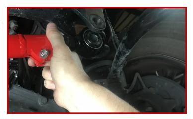
Reusing the factory hardware, place bolt into track bar bracket and install nut.
