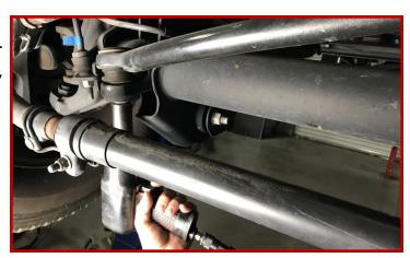
With aid of an appropriate device (i.e. Floor jack, Bottle Jack, Pole jack), apply a lifting force to bottom of the track bar ball joint. Strike side of axle track bar mount to unseat taper using a hammer/Air hammer, as pictured.
