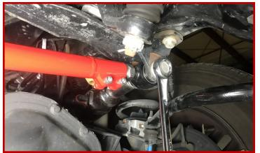
This track bar has been preset at 37", which is the length the average end-user should need.
