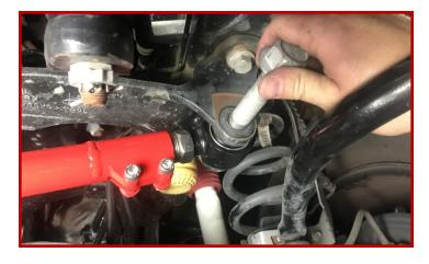
Insert ball joint into taper on the axle and start the nut.
