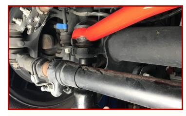
Insuring the castle nut aligns with the predrilled hole, install supplied cotter pin.
