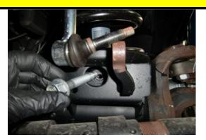
Install lower shock bolt and tighten to factory specs. Repeat these steps on the opposite side of vehicle.
