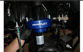
Install spacer into upper spring mount location with upper shock mount in original position. Use the hardware provided and tighten to factory specs.
