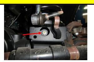
Remove end link from mount. Now you can access the lower shock bolt located under the lower spring housing.
