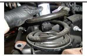
Remove bolt from shock. The nut is fixed the housing on Lower the axle to remove the shock from the mount. the other side of the shock mount.
