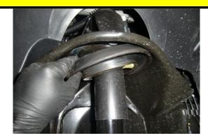
Remove upper spring isolator and set aside. It will remount under new ReadyLift T6 Billet aluminum spacer.
