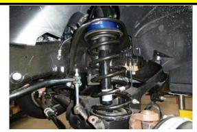
Reinstall front coil spring into original position and carefully raise axle enough to allow shock to orient in it's original position.
