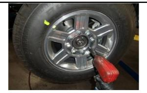
Mount wheels/tires and torque to factory specs. Lower vehicle to ground and align. Make your final measurement
