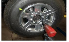
Begin by placing vehicle on level working surface and take an support vehicle on jack stands and remove front wheels/tires initial measurement.
