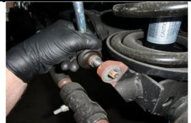
After both spacers are installed you may now attach the sway bar end links and tighten to factory specs.
