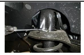
Loosen the upper shock mounts (3) nuts. This will allow Lower the axle e from the perch at from the perch at the shock to move freely, but not fall out.
