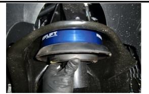
Reinstall rubber upper spring isolator under spacer as shown.
