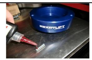
Prepare the T6-1090 spacer by applying thread locking compound to the allen set screws and tighten.
