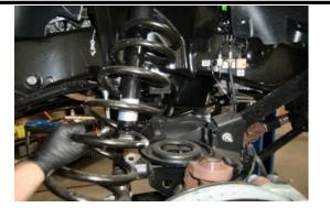
Lower the axle enough to allow the spring to be removed from the perch and out from the vehicle.
