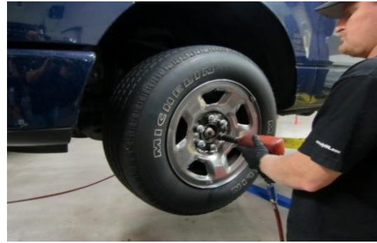
Support vehicle on jack stands and remove front wheels/tires
