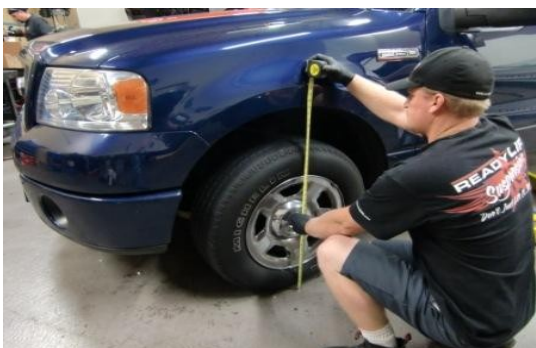
Begin by placing vehicle on level working surface and take an initial measurement.
