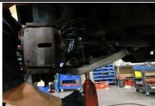
Disconnect sway bar endlinks from below on both dr./pass. side of vehicle as shown.
