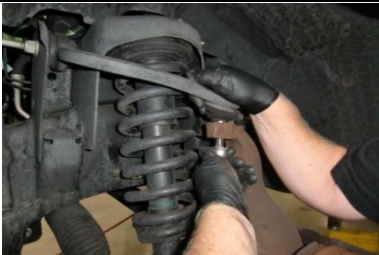
Once loose, pull down on upper control arm and remove ball joint nut.
