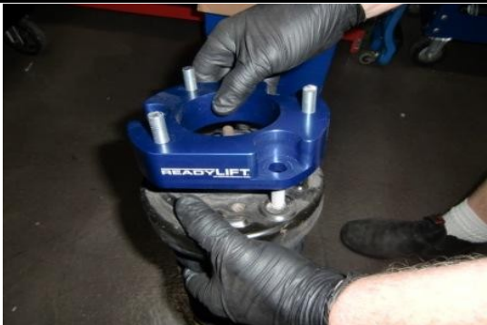
Place assembled strut extender on top of OE coil-over assembly with factory hardware.
