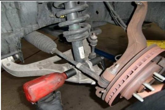
Loosen lower coil-over shock nut and remove bolt. .
