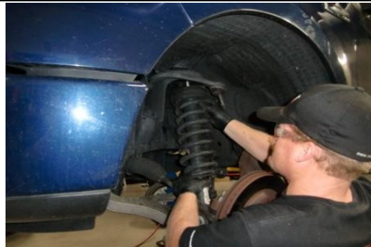
Remove coil-over assembly from vehicle.
