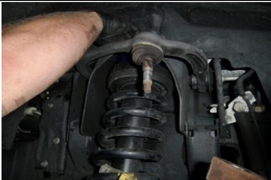
Shown here, coil-over assembly reinstalled. Attach with provided flange nuts and tighten to factory specs. 4WD models use caution not to tear outer CV boot.
