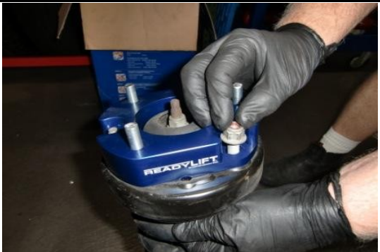
Tighten to factory specs. Note: you will be installing the entire assembly back into vehicle at 180 degrees rotation.
