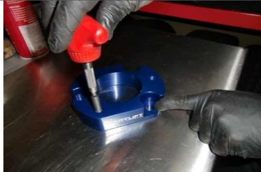
Use allen wrench or proper tool to tighten set screw studs.
