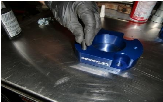
Begin assembling your T6-2058 billet aluminum extended strut extension by applying thread locking compound and installing supplied set screws.
