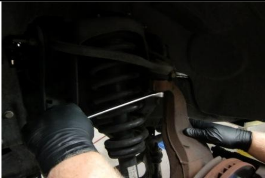
Next, loosen upper ball joint nut, but do not remove. Leave a few threads on in order to break ball joint loose.
