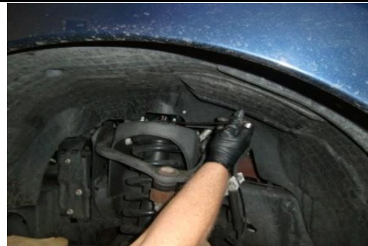
On top of coil-over mount, loosen and remove (3) nuts as shown.
