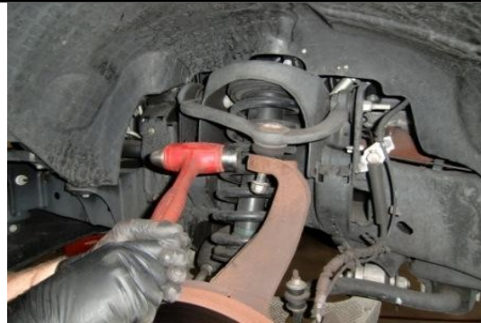
Carefully strike spindle with hammer to break ball joint loose.
