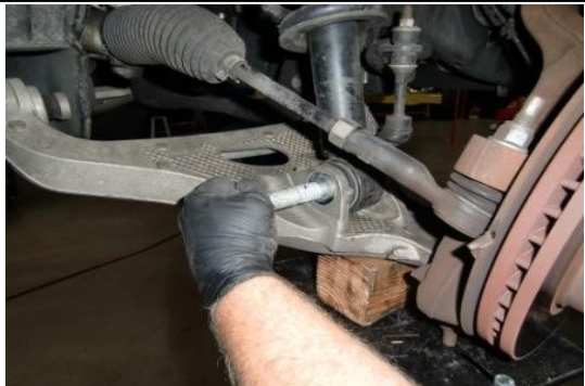
Reinstall lower coil-over bolt. You will need to raise lower control arm.
