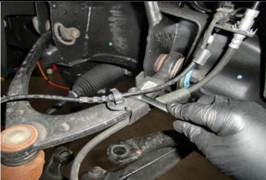
Remove ABS/brake line bracket from upper control arm.
