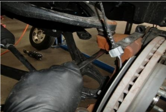
Loosen upper ball joint nut but leave a few threads engaged.
