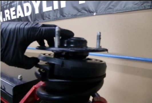
Remove upper steel mounting hat.
