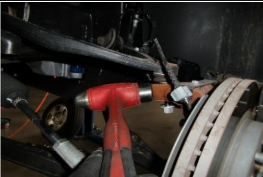
Carefully but with force strike spindle as shown to break loose ball joint.
