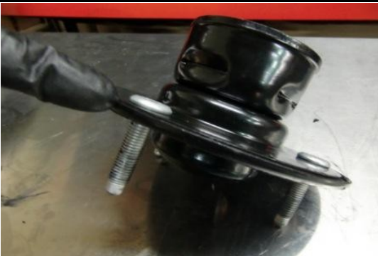
Remove (3) pressed in studs from mounting hat. They will not be reused.
