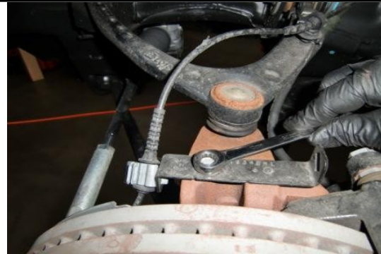
Shows removal of ABS bracket bolt on top of spindle.
