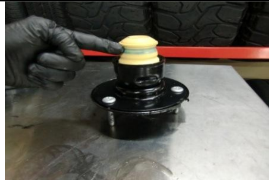
Next remove foam bumpstop from mounting hat.
