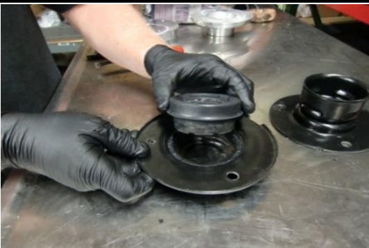
Remove inner rubber bushing as shown, it will be re-used in the T6-3085 billet extended mounting hat..
