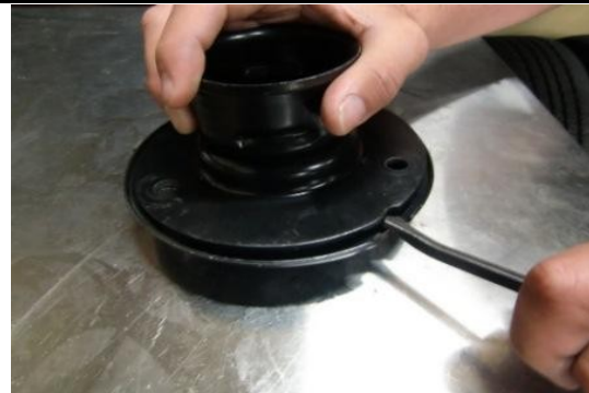
Pry two halves of the mounting hat apart to expose rubber bushing inside.
