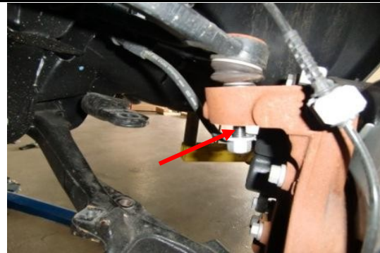
Should look like this for the next step. Note gap with nut flush with ball joint stem.
