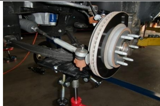
Now support suspension with floor jack or equivalent and raise slightly to remove pressure from ball joint.
