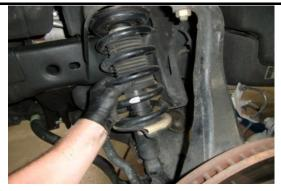
Remove coil-over assembly from vehicle. Note: 4WD models be careful not to damage outer CV boot.
