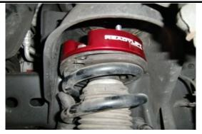
Reinstall assembly into position and attach with provided flange nuts. Tighten to factory specs.
