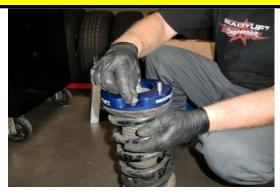
Photo: Shows factory hardware being installed. Coilover assembly will be reinstalled 180 degrees rotated.
