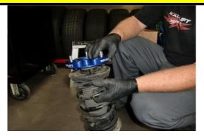
Place spacer on top of OE coil-over assembly and attach with factory hardware. Tighten to factory specs.
