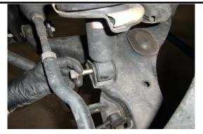
Photo, bolt removal, may be under tension, push down on suspension to loosen.
