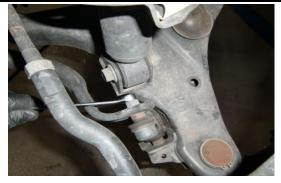
Disconnect sway bar endlinks from below on both dr./pass. side of vehicle as shown, and move bar down.
