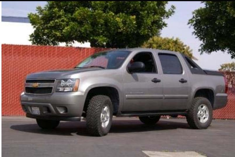
After ReadyLift® 66-3085 and 66-3010. 285/70R17 tires mounted on Factory wheels.
