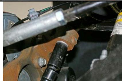
19. Return to the sway bar end link assembly and permanently tighten.
