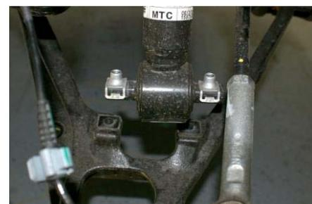
10. Remove the three upper strut nuts that secure the strut to the frame housing.
