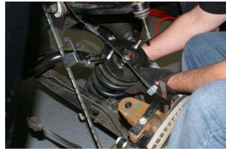
12. Install the new ReadyLift® strut extension spacer onto the top of the factory strut. Unlike some kits, you don't need to cut the studs off or swap the struts from side to side. The ReadyLift aluminum spacer is designed to provide the necessary lift while retaining the use of the factory strut studs. This is a great advantage should you ever want to return the vehicle to stock such as with a lease vehicle.
