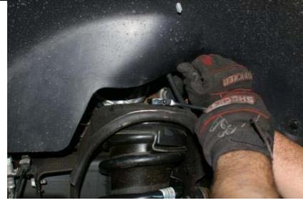
17. Reinstall the sway bar end link assembly. You will only be able to install the nut onto the end link bolt. You will have to tighten it once the spindle has been re-attached to the ball joint and control arm.
