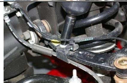
5. An 18mm socket is used to loosen the upper ball joint nut. The nut should remain on the ball joint stem.
